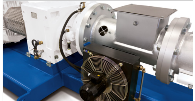
Drive with combined gearbox-bearing assembly
